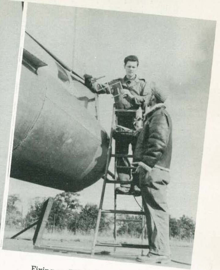
Fixing a flak hole — Station 131
