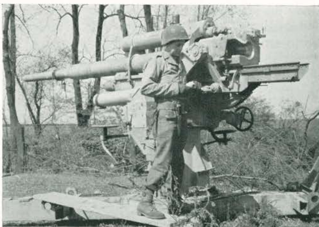
In their task of reduction of the Ruhr industrial area, XVI Corps troops were faced with 88mm. high-velocity weapons such as this, once used for anti-aircraft defense of the area and later turned against the assaulting ground forces.
