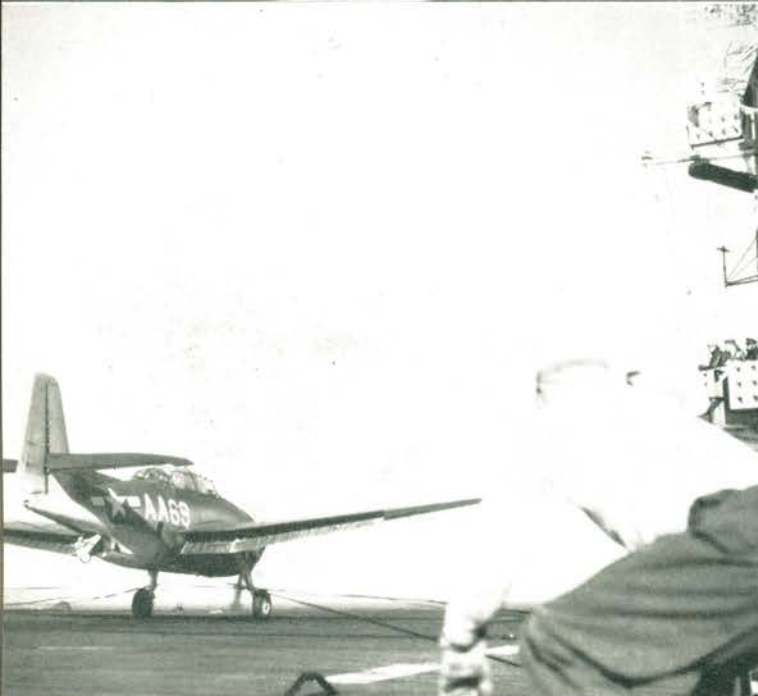
LANDING GEAR CATCHES BARRIER CABLE
