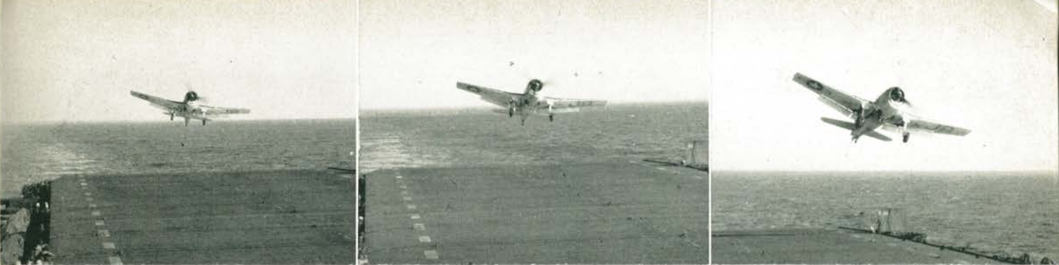
POOR APPROACH, NO LANDING
