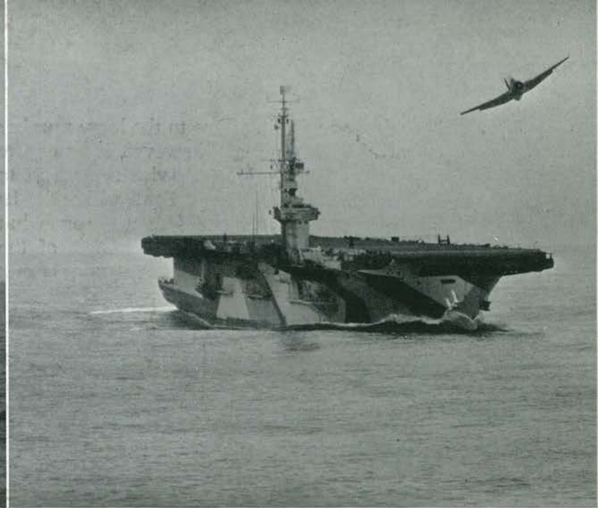
Lunga Point noses into a ground swell as she turns into the wind preparatory to recovering planes.
