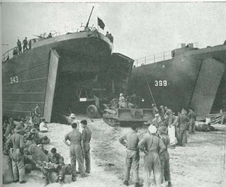
CATSKINNER. J. B. McLelland backs his loaded carryall through the yawning doors of LST 343. Heavy equipment went on the well deck, while trucks and jeeps were parked topside. Frank Keker (left foreground) calmly reads "Superman."
