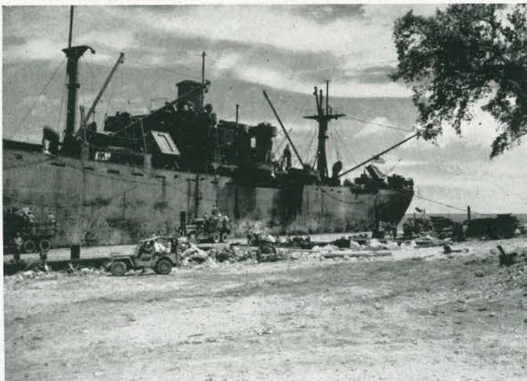
FIRST LIBERTY SHIP unloads at Stirling Dock on 30 January 1944. Pier was 428 feet long and 43 feet wide, so all holds of ships could be worked simultaneously. Seabees furnished winchmen and the signalmen while Kiwis unloaded cargo into trucks.
