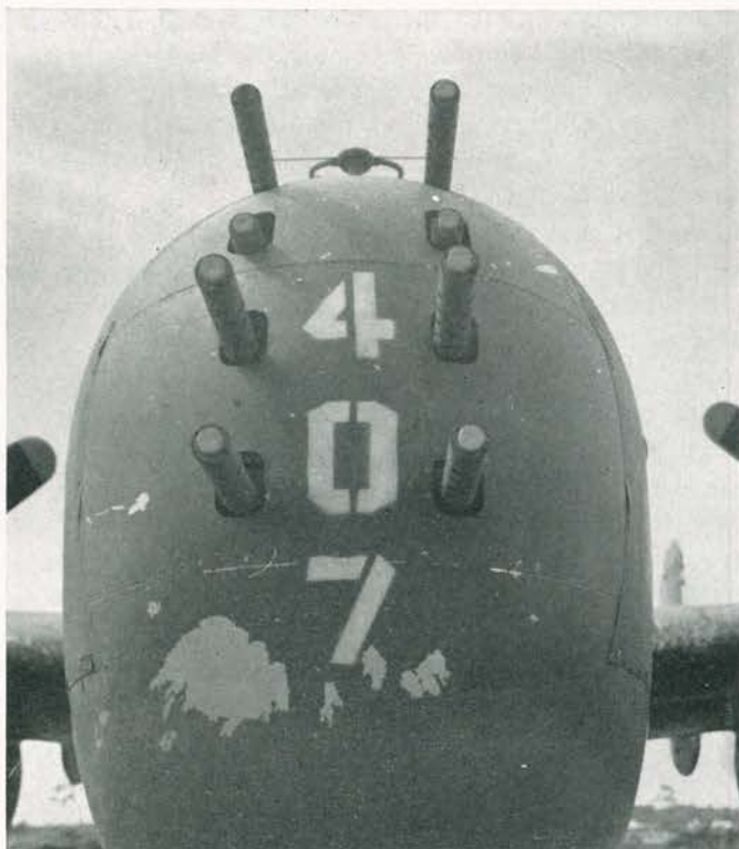
Sudden death in eight efficient packages. The nose armament of the B-25J2
