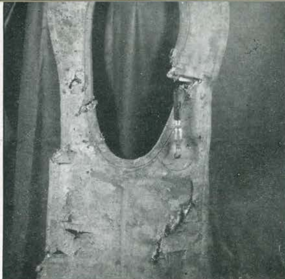
The waist gunner's Mae West. He was wearing his flak suit under it, and although the metal plates were bent and broken, none was penetrated. The gunner escaped with foot and leg wounds.
