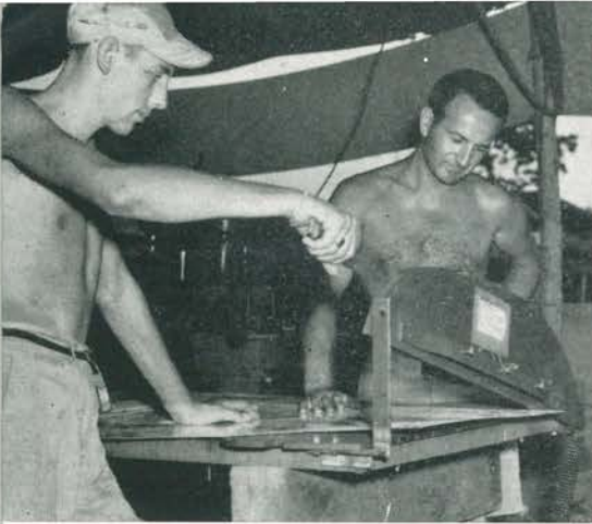
A couple of proud inventors demonstrate the sheet metal cutter they devised from some old armor plate, a spring, and a few nuts and bolts. Very superior to shears.
