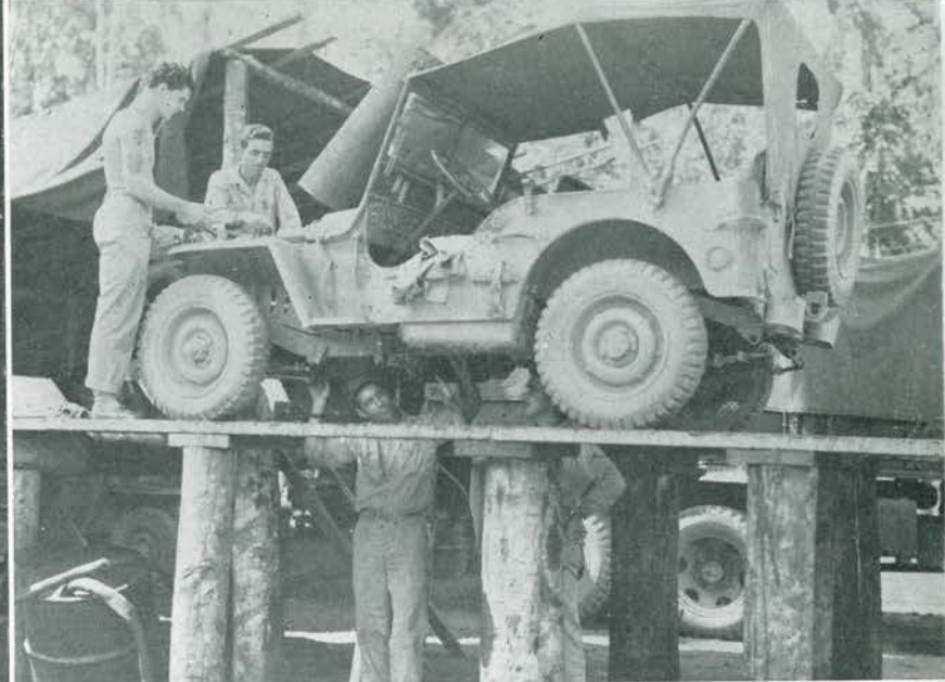
The grease rack at your corner filing station is probably prettier, but Transportation in New Guinea kept them rolling with a rack like this.
