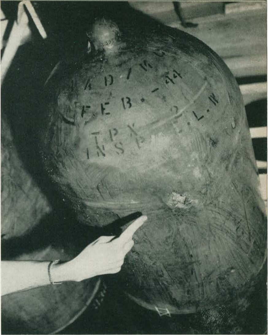
Shrapnel damage to warhead.
