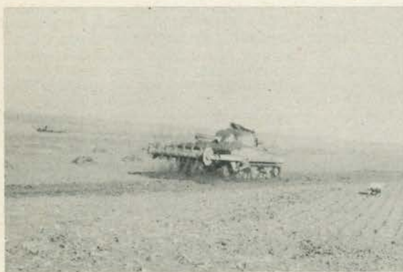
"Flail tank" in use in "B" Company mine clearance
