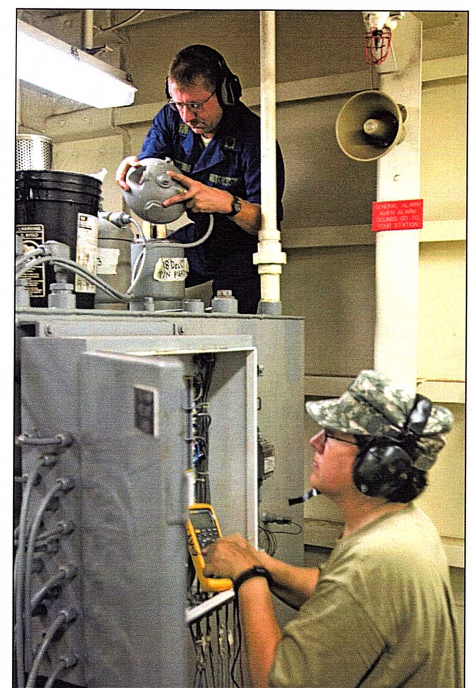
Chief Warrant Officer Vicky Lipps, the first engineer (bottom right), and the Chief Engineer John T. Owens II both with the 548th Transportation Detachment struggle to fix a power glitch in the Kuroda's hydraulic wench anchor system in the bow thruster room of the ship. (Top) Owens changes filters that were melted by hydraulic fluid.
