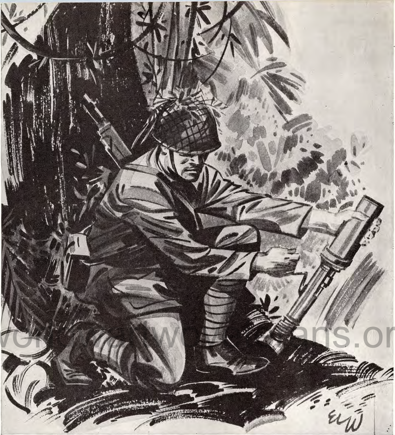
JAP 'KNEE' MORTAR , which became famous throughout world, is fired by enemy soldier. Actually mortar is spring-actuated grenade thrower, and is fired from the ground, not the knee. Latter fallacy resulted from mortar's curved baseplate.
